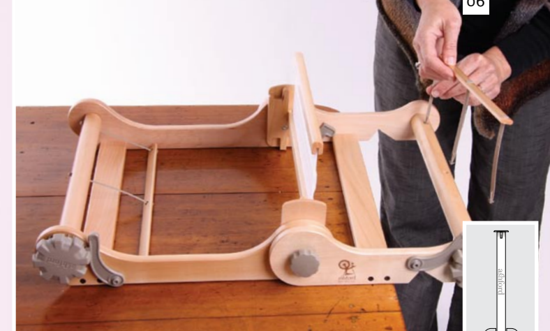
Now push the arrowhead ends into the wide flat edge on the back and front rollers.
