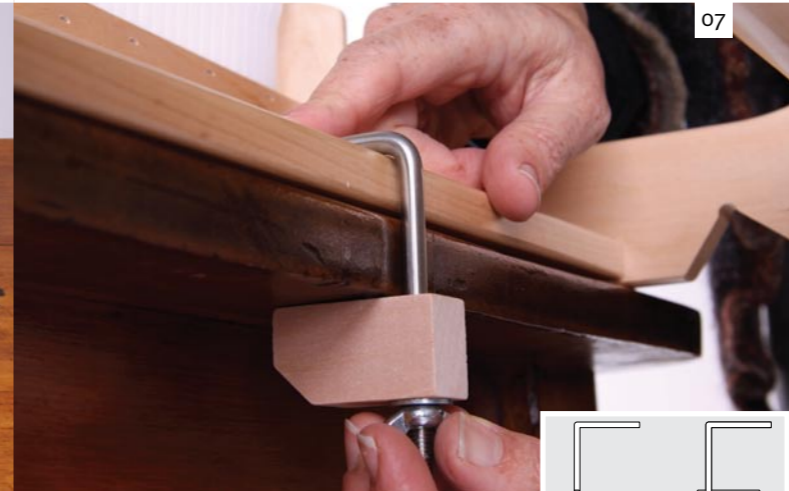
Assemble the clamps. Clamp the back of the loom to the table.
