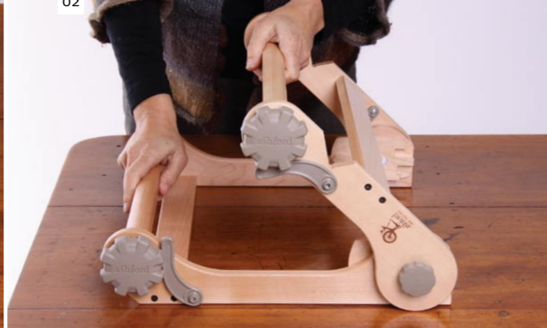
Loosen the side knobs and unfold the loom.
