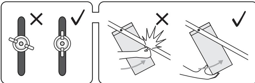
lift the bottom of the castle again and allow it to fold down completely. Then insert the knobs back through the slot and into holes near the top of the castle side and tighten. This will ensure the castle is well supported when transporting the loom.
