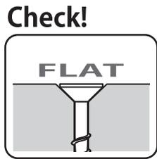
Attach the bottom cross rails to the bottom of the castle sides with 30mm (1¼") screws. Check! Only use 30mm (1¼") screws. Longer screws may damage the sides.
